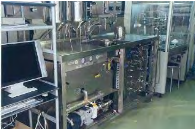
UHT/HTST 杀菌系统(供液体无菌填充用) UHT/HTST Lab-25HVH Sterile System (MicroThermics, Inc.)
