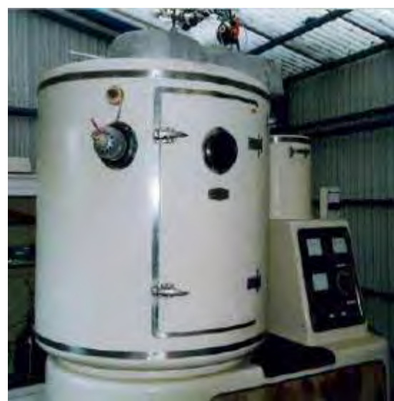
喷雾干燥机(丹麦制) Spray Drier, Anhydro ,Danish
